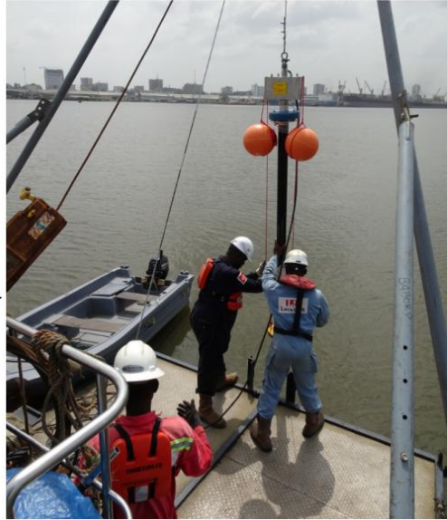
Core Sampling from a small survey boat
